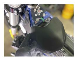
4) Behind the left tank shroud is a black protective panel mounted to the frame. At the top is a single T27 Torx screw that needs to be removed.
