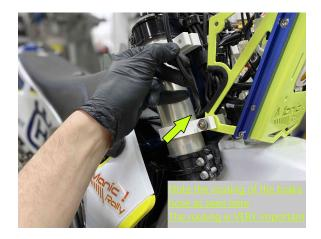
17) Now the fairing assembly can be mounted on the bike, but before proceeding ensure that the front brake hose is placed ABOVE the lower right sidle fork mounting clamp! The brake hose CAN NOT be routed beneath this mount! Hold the fairing with the lower mounting holes in-between the lower fork mounts while inserting (12) of the (4) M6 cap Allen mounting
