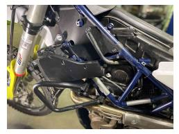
3) On the front "tank shroud" there are (2) top and (2) front T27 Torx screws that need to be removed. After this the left hand side panel can be removed and set aside.
