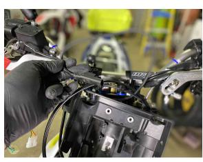
11) You can now pull the handlebar control cables on the left and right side through the top OEM plastic dash holes. Place the extracted cables on top of the handlebar controls to keep out of the working area and pay SPECIAL ATTENTION to keep the ABS / speed sensor pickup somewhere it can not be cut or damaged!
