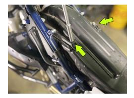
5) Nestled between the frame you will find the air box intake snorkel lid. Remove the (2) 8mm head screws to remove the snorkel lid and set aside. Ensure that the air filter is not removed!
