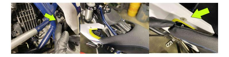
1) Pull seat release loop under left side of bike to release rear of seat then pull out front seat affixing pins on left and right on front of the seat. The seat can now be removed completely and set aside.
