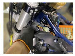
6) Underneath the lock cylinder you will find the (2) electrical plugs circled here which must be disconnected. Once disconnected you can gently bend back the left side frame cover panel and pull the wires free of the frame. Pay attention to how the wires are routed as they will be replaced later.
