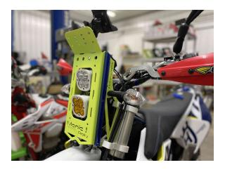
19) Provided the wiring is organized and fastened well you can now tilt the fairing upright and place the last (2) top mounting m6 cap bolts with rubber backed washers. Once all (4) cap bolts
