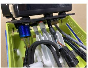
16) Now place the ADV-Light fairing assembly on a scratch free soft work surface. You can Remove the remove the windscreen assembly temporarily (not completely necessary) be removing the (2) M5 screws
