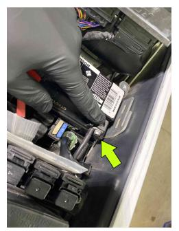
2) Under the seat you will find the bikes ECU held in place on 2 sides by a rubber strap. Pull up on the strap at the pins to release
