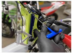
20) There are (4) LED light tightening screws with (2) on each side. These can be loosened slightly so the lights can be tilted for adjustment. These screws should NOT need to be excessively
