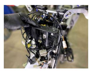
10) Remove any other connected electrical plugs at this time and take whatever steps necessary to note / remember all mating plug pairs if necessary. Remove the front brake line and ABS / speed sensor pickup from the OEM plastic dash keeper then the (2) 8mm bolts affixing the dash. Gently pull the dash away from the triple clamps.
