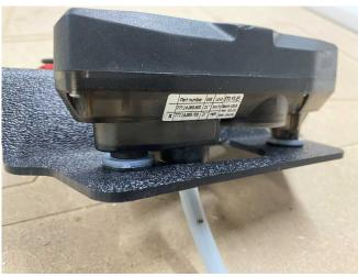
6) To remove the turnsignal indicator from the factory bracket simply push it out of its hole. Now install it into the rubber grommet on the dash plate; this step can be aided with a dab of water with dish soap to help the indicator lamp into place
