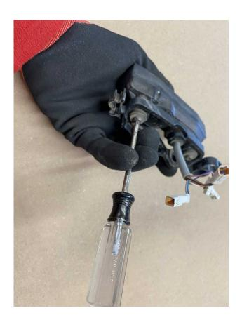
3) Now you will remove the key lock cylinder from the OEM headlight mask and attach to the ADV-light body. Taking care not to deform or "mar" the aluminum nut, use a set of channel locks to loosen the aluminum knurled retaining nut on the top of the lock cylinder. Fully un-thread and remove from the headlight mask. Place the included O-ring onto the lock cylinder before proceeding!
