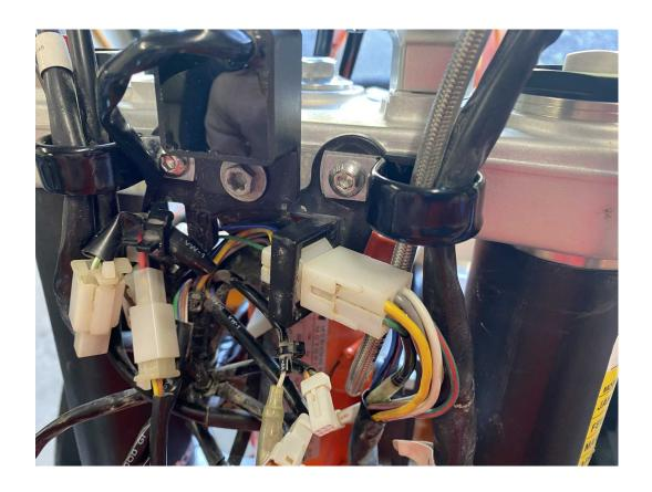
8) Now the included plastic fork clamps can be installed. Make sure the plastic clamps are "warm" before preceding! Installation requires the clamps to bend / flex and at a temperature of less than 60deg F they could tear or crack. Once installed the clamps work in tension and are incredibly strong. There is also NO NEED to flex the clamps open before installation!
