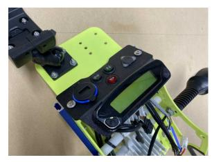
10) Now the fairing assembly can be mounted on the bike. Before proceeding it might be a good idea to place a dish towel over your front fender to protect from possible scratches.
