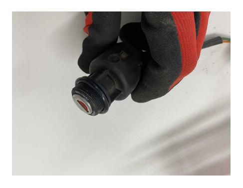
4) Place the lock cylinder into the hole on the right lower side of the ADV-light fairing body and re-install and tighten the aluminum nut to a suitable torque. Be careful not to over-tighten which could remove the threads from the plastic lock cylinder but do not leave loose. The O-ring should create constant pressure and reduce the chance of the nut loosening and being lost.
