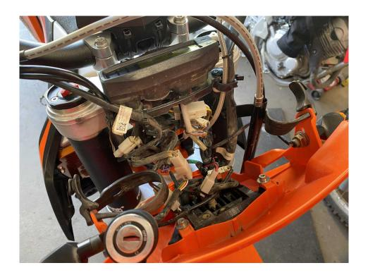
2) Under the factory speedometer there are (2) T-20 screws that will need to be removed (pictured off the bike here). Before removing speedometer, carefully disconnect the electrical plugs connecting the speedometer to the factory wiring loom with a fine tip electrical pick. Remove the speedometer and set aside then the (2) 8mm hex bolts attaching the speedometer bracket to the top triple clamp.
